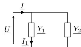
$$\begin{cases} \underline{I} = (\underline{Y}_1 + \underline{Y}_2) \underline{U} \\ \underline{I}_1 = \underline{Y}_1 \underline{U} \end{cases} \quad \text{donc} \quad \boxed{\frac{\underline{I}_1}{\underline{I}} = \frac{\underline{Y}_1}{\underline{Y}_1 + \underline{Y}_2}}$$
