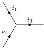
$$i_1 + i_2 = i_3 \quad \text{donc} \quad \underline{I}_1 + \underline{I}_2 = \underline{I}_3$$
