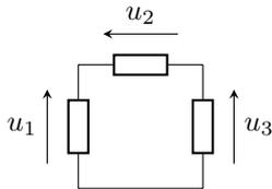
$$u_1 = u_2 + u_3 \quad \text{donc} \quad \underline{U}_1 = \underline{U}_2 + \underline{U}_3$$
